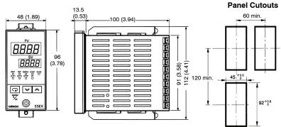
Note: 1. Recommended panel thickness is 1 to 8 mm.
