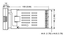
1. Recommended panel thickness is 1 to 5 mm.
