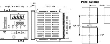
Note: 1. Recommended panel thickness is 1 to 8 mm.
